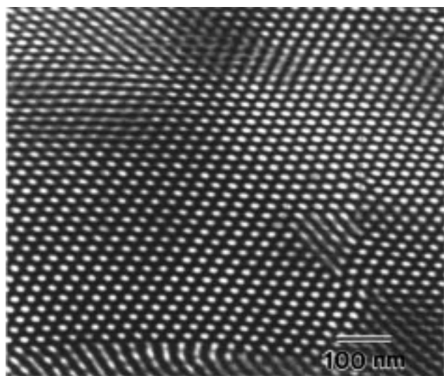
Figure 3. TEM micrograph of the SIS31 copolymer/hPI blend revealing the existence of dispersed styrene-rich cylinders in an isoprene matrix. This morphology persists from 31 to 27 vol % styrene. The neat SIS32 copolymer, characterized in detail elsewhere, 32 possesses the G morphology.
